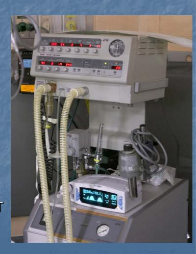
Infra-red spectrography CO<sub>2</sub> absorbs specific wavelengths IR light • Amount absorbed  $\propto$  concentration Interference Atmospheric pressure CO2 Molecules  $\Box 0_{2}$ Water vapor
